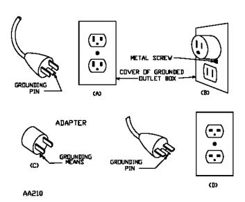
This appliance must be grounded. In the event of malfunction or breakdown, grounding provides a path of least resistance for electric current to reduce the risk of electric shock. This appliance is equipped with a cord having an equipment-grounding conductor and a grounding plug. The plug must be plugged into an appropriate outlet that is properly installed and grounded
